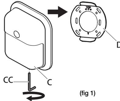
2. Route the junction box wires through the large center hole in the mounting plate (D).
