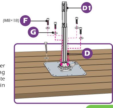
Use **1/4 inch** -diameter galvanized/stainless lag screws to mount the plate
