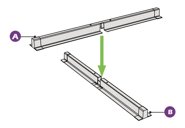
Place the part A upper crossbar on the part B lower crossbar. Then, put the base weights on the cross bars.
