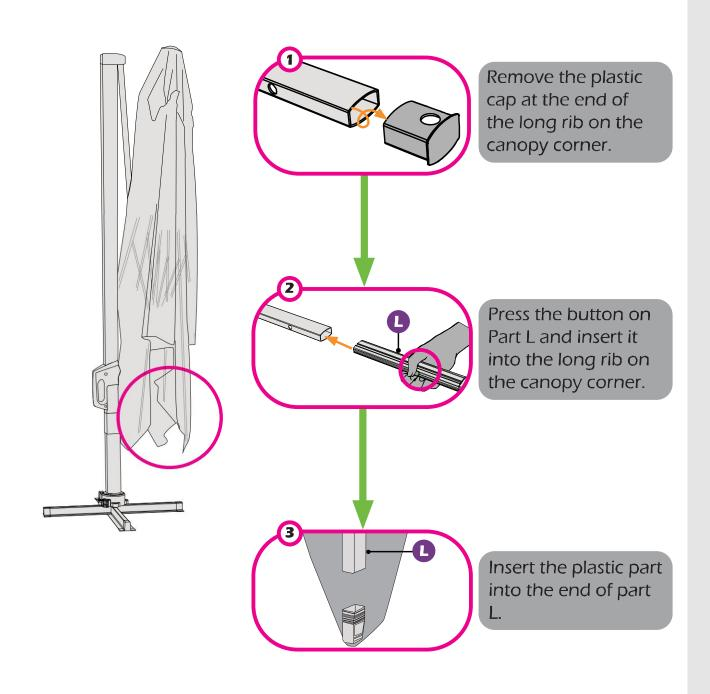
Repeat the above steps to finish the installation of other three parts L.
