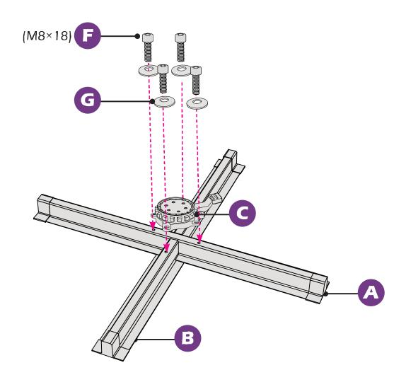
Attach the rotating part C to the cross base with four part F screws and four part G washers.
