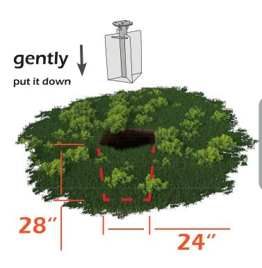
Dig a hole roughly 28" deep and 24" across. Gently put the inground base in the hole and make sure it is level before backfill the hole with concrete.
