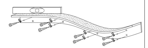
With screw cap over screw, insert all screws into wall beam studs. Tighten all screws then snap close screw caps.
