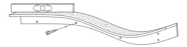
Use screw head to mark where ever wall anchors will be placed. Reminder, recommended shelf installation into at least 2 wall studs.
