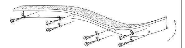
Carefully rotate shelf upward so shelf is level. Insert rest of screws into wall anchors and into wall beam studs. Tighten all screws then snap close screw caps.
