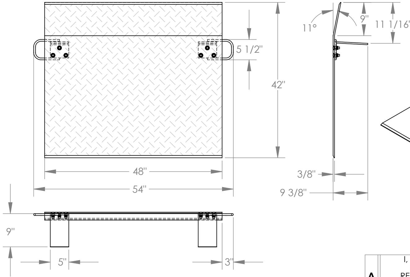
NOTE: BEND OR CROWN IS 11° AND LOCATED 9" FROM EDGE OF DOCKPLATE
