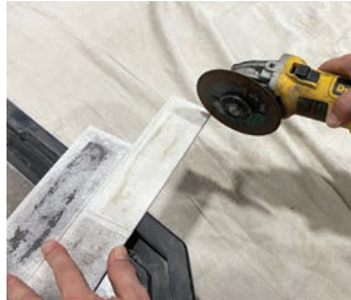
Using a mason wheel on a 4" grinder to cut notches or more detailed cuts.
