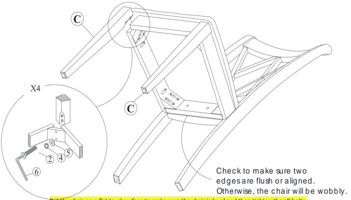
Put the chair on a flat level surface to make sure the chair is level and then tighten the all bolts.
