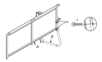
2. Connect the left arm (Part C) to the back (Part A) using Bolt (J) as indicated in the diagram.
