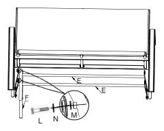
6. Connect the left leg (Part G) to the glider (Part E) using Screw (L), washer (N), and Plastic washer (M) as shown in the diagram.
