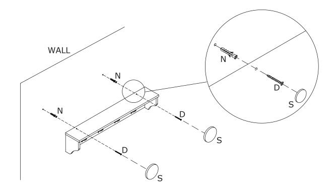
Drill holes on your wall, knock into part(N). Fix the component(assembled in step 3) to wall using screw(D) as shown. Use sticker(S) to cover screw(D).
