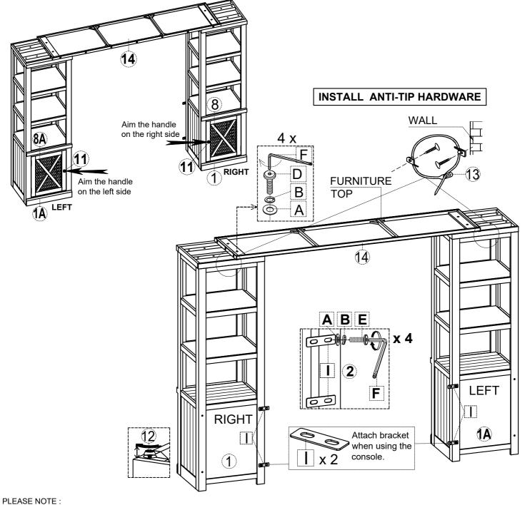
This assembly will require two people. To help prevent the possibility of tip-over, install the ANTI-TIP hardware restraints provided.
