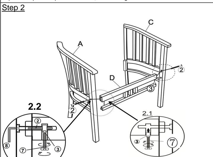
Insert the tenons on Leg Support Bar(D) into the mortises on Left Arm Panel(A).
