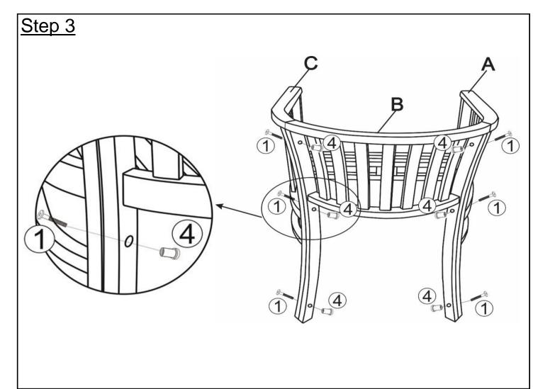
Attach Backrest Panel(B) to Left Arm Panel(A) and Right Arm Panel(C) using Bolts(1) and Sleeve Nuts(4) with Allen Keys(8).
