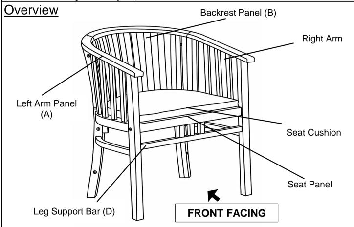
This Armchair has multiple parts and may require up to 30 minutes to assemble. To give you an overview of the Armchair parts, the above picture is to help you put the various parts into perspective. Please read through the instructions below to familiarise yourself with the parts and steps before assembly.
