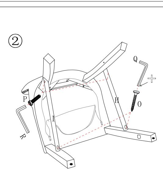
Caution: The bars H and I should be in horizontal position after installation. If not, the most possible reason is the rear feet were not installed correctly.Please check and swap the left and right rear feet.
