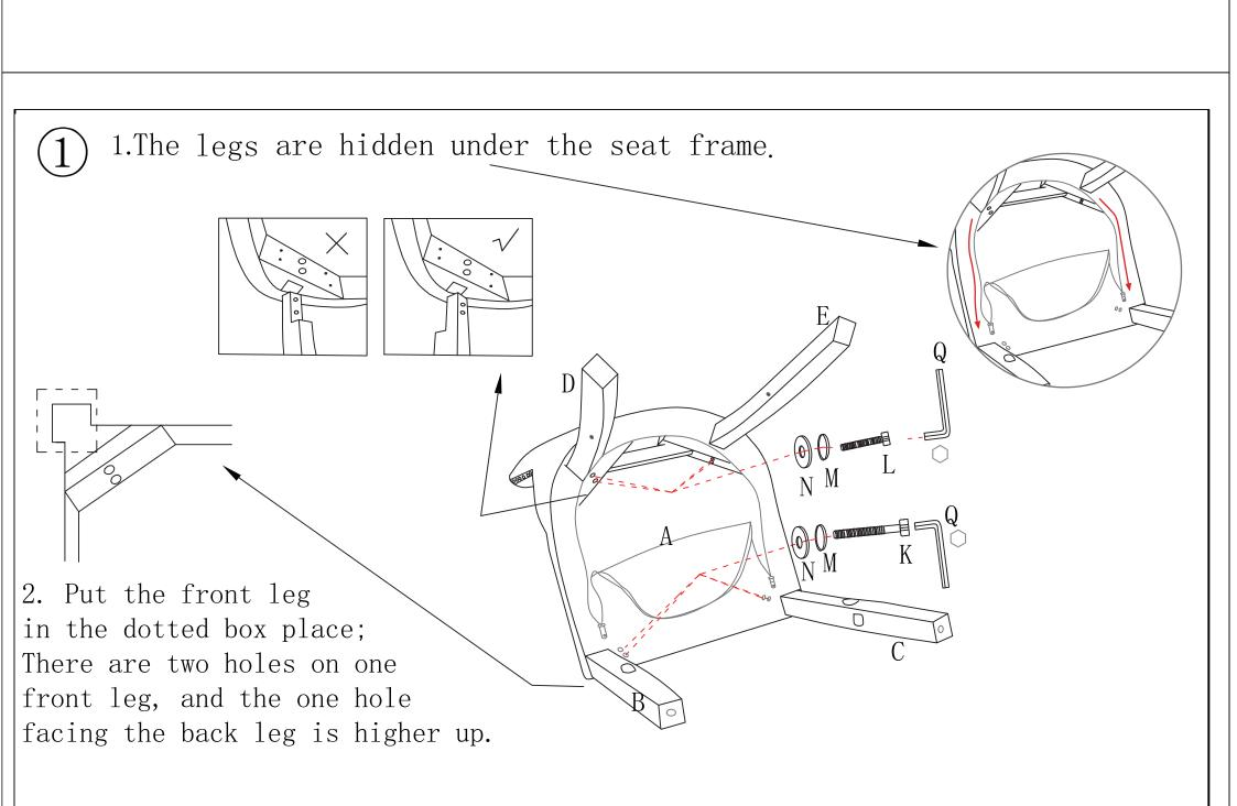
3. Tighten all the screws to 80% of maximum tightness.
