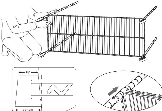
**4** Push the bottom shelf down onto the plastic clips until the shelf fits tight.
