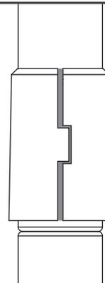
3. The end with a notch is downward, which is designed to help determine the direction of the wire shelf. At the same time, according to the text and indication signs on the shelf and clips, you can confirm the correct installation steps.
