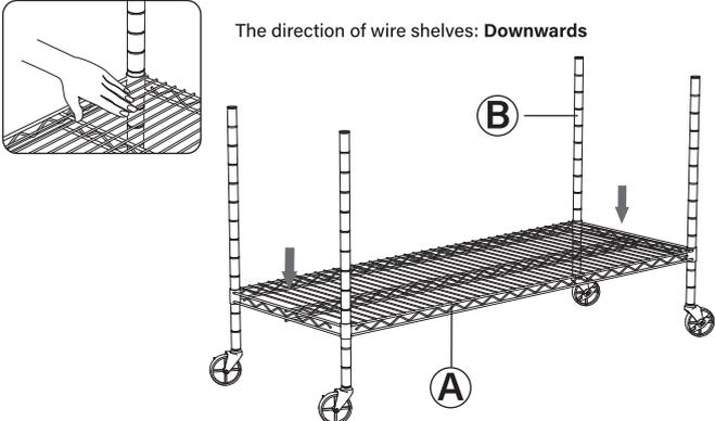
**5** Install middle tubes/top tubes accordingly.
