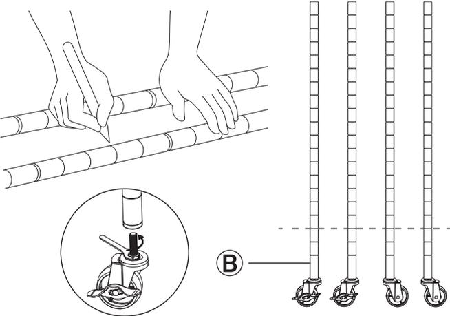
**2** Place the clips onto the marked groove locations.
