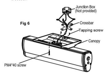
8. The unit can be installed on any surface, you may rotate the EXIT panel in any angle from 0° to 180°, ceiling mounting rotate 90° become wall mounting.
