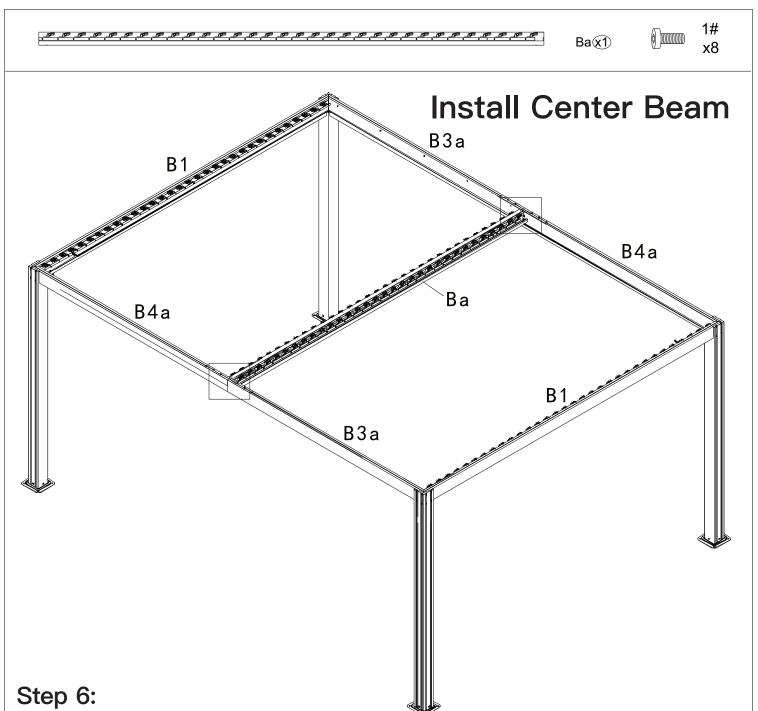
Install Part Ba to the middle joint of Part B3a and Part B4a With 4 Bolts 1# as shown. Repeat the above procedures to assemble another side.
