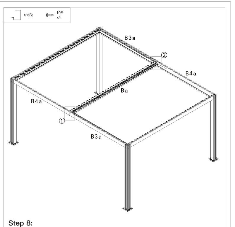
Install Part #G2 at the joint of Part #B3a and Part #B4a with 4 bolts 10# as shown.
