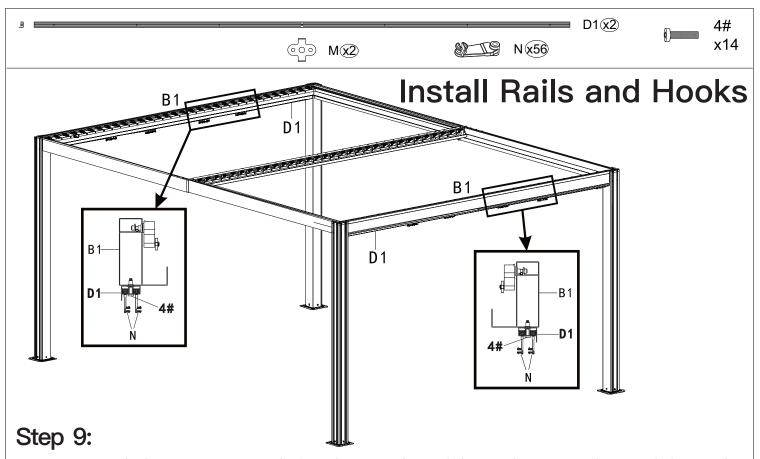
Fix Part #D1 below Part #B1 with 6 Bolts 4#; Then slide Hooks #N to the inside&outside
