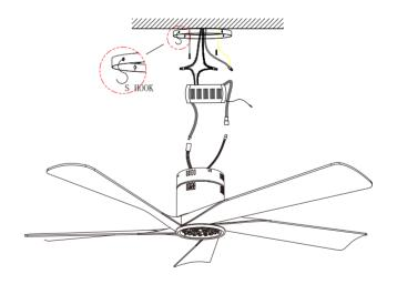
Position the fan blade in order ,Turn the screw until it's tight
