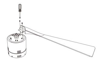
3. Line up the 3 Metal Plate with the screw, snap it in place, and then tighten the screw. And than use the screws to attach the 4 LED light plate to the 3 Metal Plate
