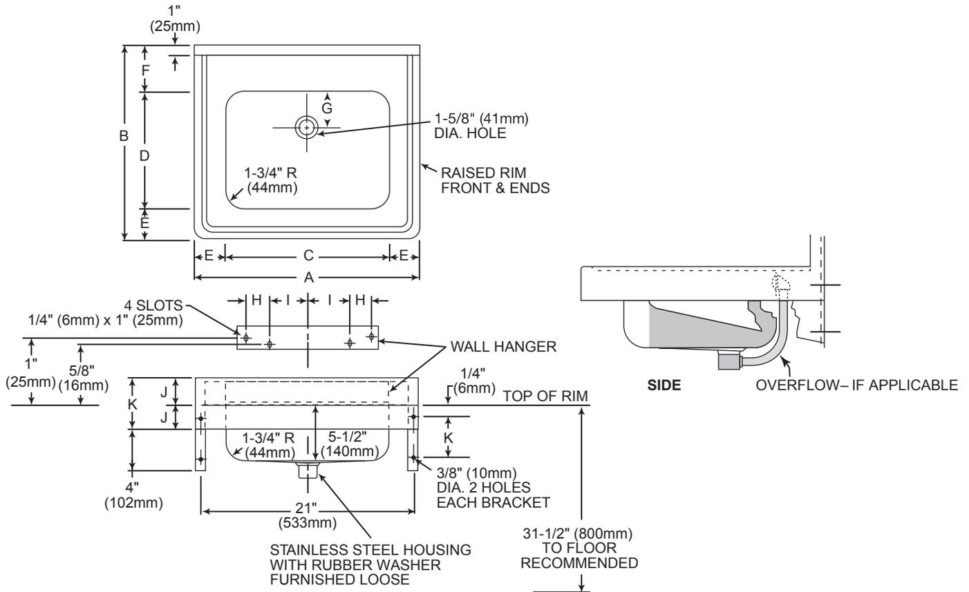
**HOLE DRILLING CONFIGURATIONS**
