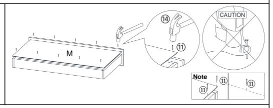
Attach Drawer Bottom Panel(M) to Drawer Assembly using Nails((11)) with Hammer((14)).
