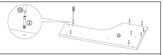
Attach Cam Bolts(2) to mounting positions on Left Side Panel(D) with Screwdriver(13).
