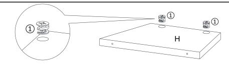
Insert Cam Locks(①) into mounting positions on Center Panel(H) by hand.
