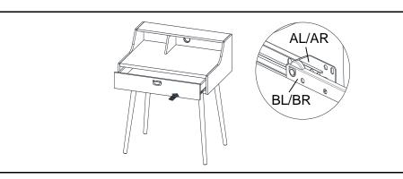
Put Drawer Assembly in place by aligning the rails.
