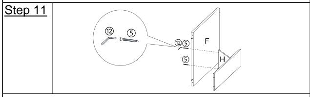
Attach Center Panel(H) to Top Panel(F) with Cap Wood Screws(⑤) using Allen Key(12).
