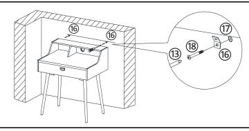
Attach Metal Brackets(16) to Wall Plugs(17) using Wall Plug Screws(18) with Screwdriver(13).
