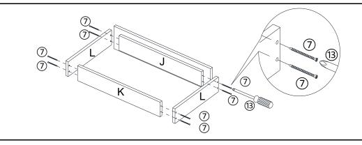
Attach Drawer Side Panels(L) to Drawer Front Panel(J) and Drawer Back Panel(K) using Screws(7) with Screwdriver(13).
