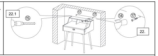
**22.1)** Drill two holes on wall at same height as Metal Brackets(16) with Power Drill(15).
