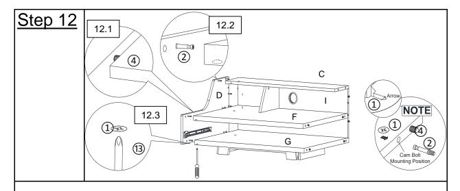
**12.1)** Insert Positioning Dowels(4) from Top Panel(F), Bottom Panel(G) and Back Panel(I) into mounting positions on Left Side Panel(D).
