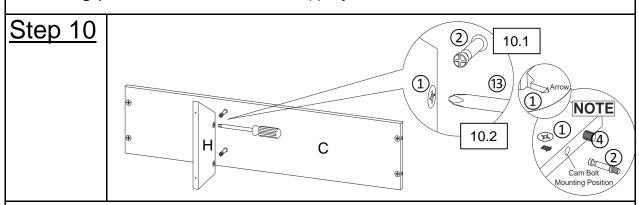
Note: Ensure the arrows on Cam Locks head points towards the Cam Bolt mounting positions.
