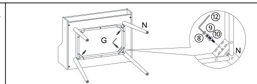
Attach Legs(N) to apron on Bottom Panel(G) using Screws(®), Spring Washers(®) and Washers(®) with Allen Key(12).
