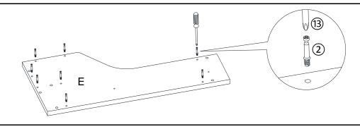
Attach Cam Bolts(②) to mounting positions on Right Side Panel(E) with Screwdriver(③).
