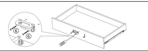
Attach Steel Handle(O) to Drawer Front Panel(J) using Screws(6) with Screwdriver(13).
