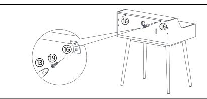
Turn the Office Desk so the back faces you. Attach Metal Brackets(16) to Back Panel(I) using Pan Head Screws(19) with Screwdriver(13).
