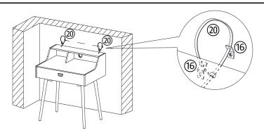
Move the Office Desk back against wall. Pull the Restraint Straps(20) through the Metal Brackets(16) on the wall and Bookcase one by one, and pull the Restraint Straps(20) tight.
