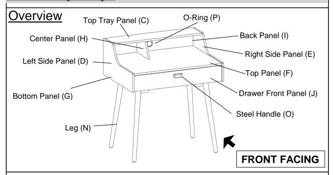
This Office Desk has multiple parts and may require up to 60 minutes to assemble. To give you an overview of the Office Desk parts, the above picture is to help you put the various parts into perspective. Please read through the instructions below to familiarise yourself with the parts and steps before assembly.
