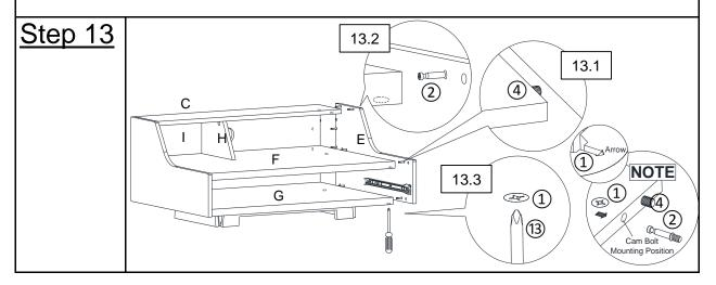
**13.1)** Insert Positioning Dowels(④) from Top Panel(F), Bottom Panel(G) and Back Panel(I) into mounting positions on Right Side Panel(E).
