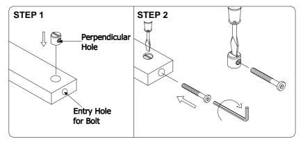
Insert Barrel Nut with the perpendicular hole facing and in-line with the drill hole that the bolt is to be inserted.
