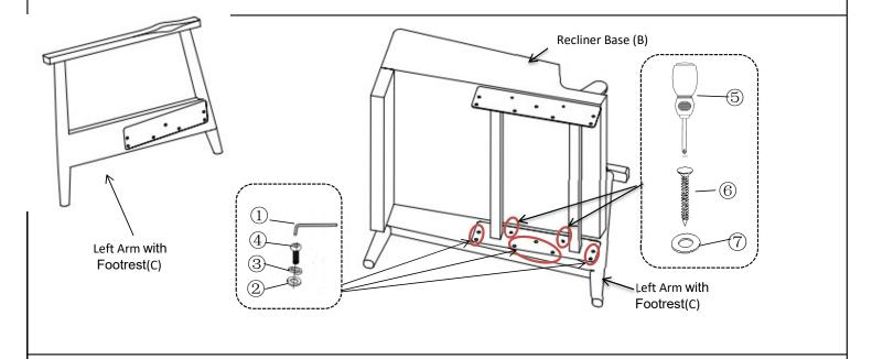
Take out the Left Arm with Footrest (C) and Right Arm with Footrest (D) from the non-woven bags. Attach the Left Arm with Footrest (C) to the Recliner Base (B) using the Bolts(4), Spring Washers(3) and Washers(②) with the Allen Wrench(①). Also use the Self-tapping screws(⑥) and Spring Washers(⑦) with the Cross Screwdriver(⑤) where indicated in the above picture.
