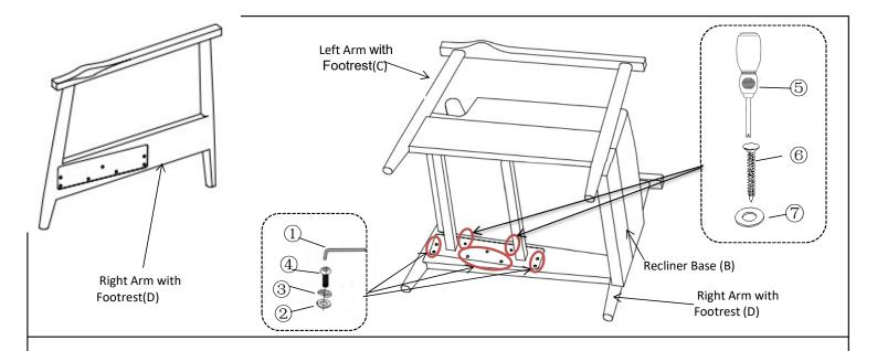
Repeat the same steps to install the Right Arm with Footrest (D) to the Recliner Base (B). Use a Self-tapping screw(⑤) and Spring Washer(⑦) with the Cross Screwdriver(⑤) to lock the remaining 2 holes
