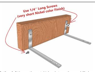
**Optional a)** Line up the metal L-brackets on the pre-drilled holes at the bottom of the small box. You need to screw it in using **% inch screws** (very short Nickel color finish)
