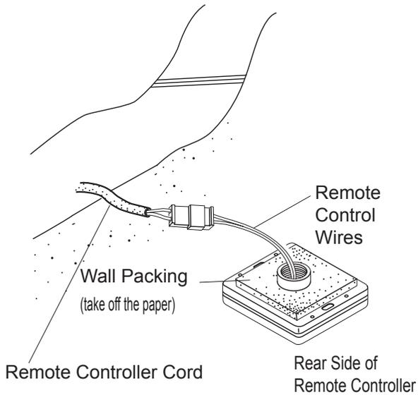
3. Remove the cover of the remote control, mark the location of the screw holes, and drill holes for the wall anchors.
