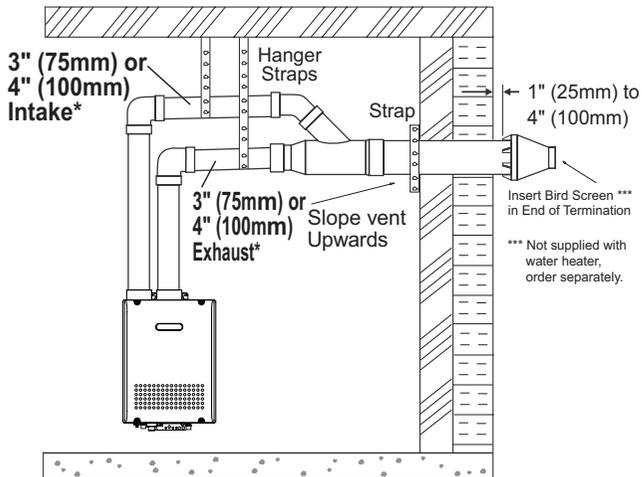
\* 4" (100mm) pipe requires the use of a reducing coupling just prior to the termination.
