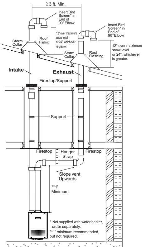
When choosing intake and exhaust terminations, you must use the same type of elbow (i.e. both 90° elbows). This will help with proper combustion by putting both terminations in the same pressure zone.
