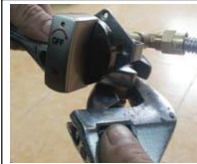
Remove propane pipe
