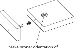
Make proper orientation of CAM LOCK when inserting CAM PIN
