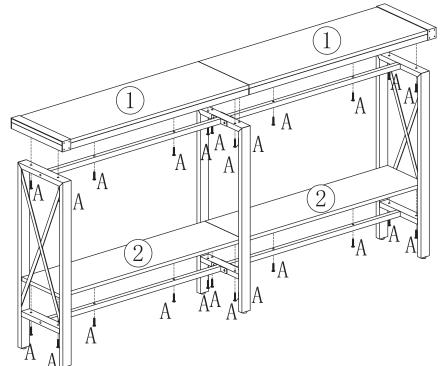
Twist screw A to connect part 1, 2 with the table leg.
