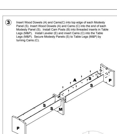
NOTE: The arrow on the face of the Cam (C) should point towards the Cam Post (B) for proper alignment.
