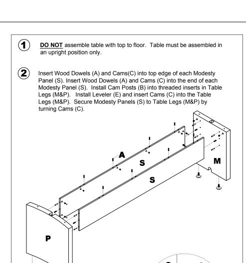
NOTE: The arrow on the face of the Cam (C) should point towards the Cam Post (B) for proper alignment.
