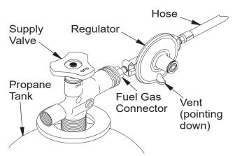
Figure 3 - Regulator With Vent Pointing Down
