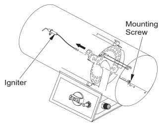
Figure 9 - Removing Igniter Mounting Screw and Igniter
