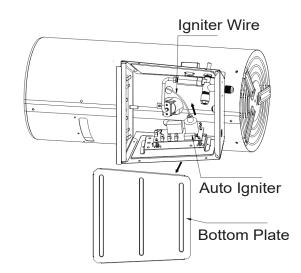
Figure 8 - Removing Igniter Wire from Igniter
