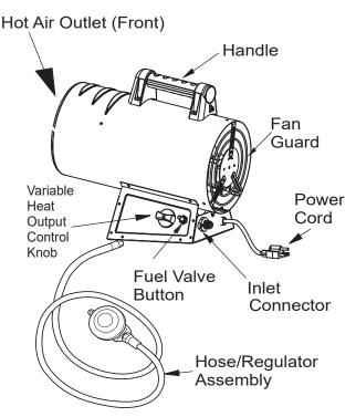
Figure 1 - Variable 60-125,000 BTU/Hr (heater may vary from illustration)
