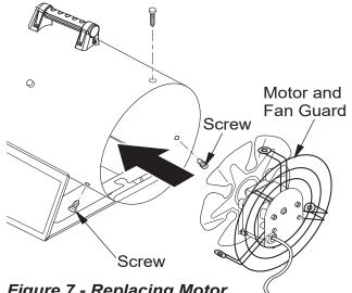
Figure 7 - Replacing Motor
