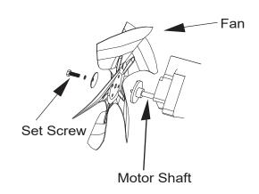
Figure 6 - Fan, Motor Shaft and Set Screw Location
