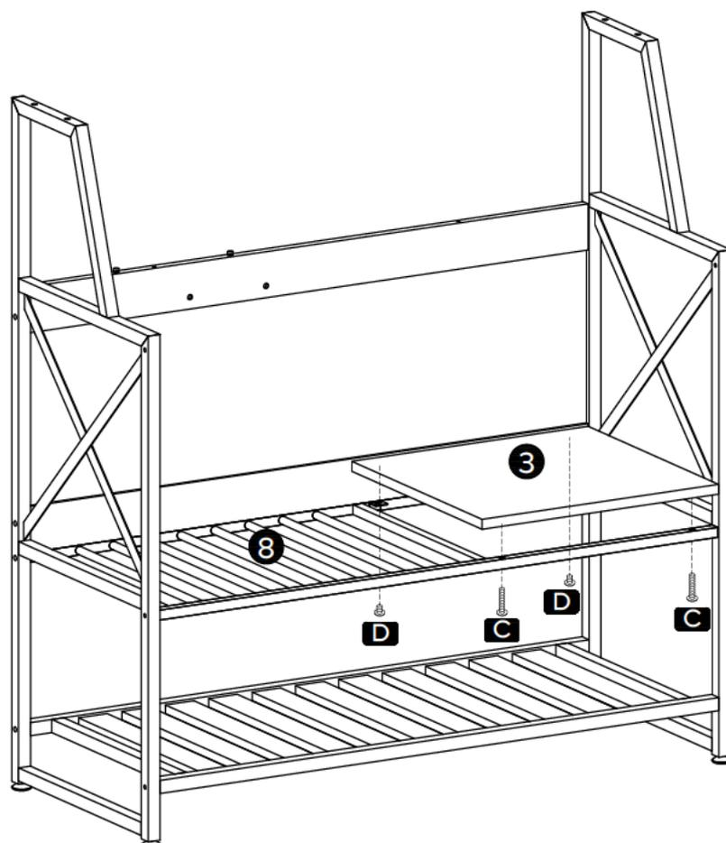
※Please be careful not to install screws C and D in the wrong position, otherwise the board will be damaged.
