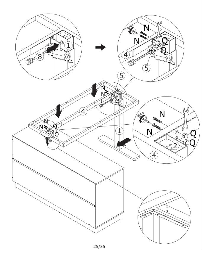
Turn the rod clockwise to tighten it, and then connect power cable 7 and 11 to control part 10 as shown.
