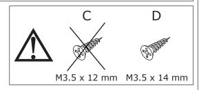
Assemble door 18 to panel 15 and 16 by fixing hinge with screw(D) as shown.
