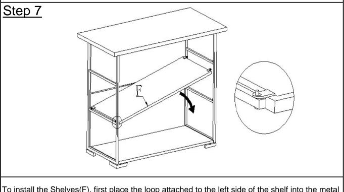
To install the Shelves(F), first place the loop attached to the left side of the shelf into the metal peg on the inside of the Left Side Panel(B) as shown in the picture above. Then lower the right side until the loops fit into the pegs on the right side.
