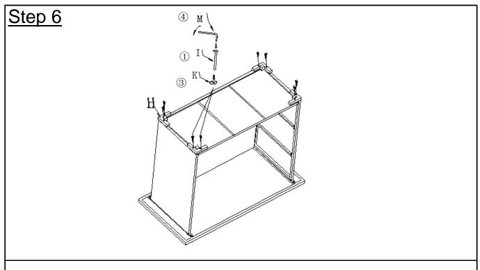
Attach the Feet Cap(H) to the Bottom Plate(G) using hardware((3, 1)) with Allen Key((4)). Now, in a gradual and sequential manner, **proceed to fully and securely tighten all Bolts at all joints.**
