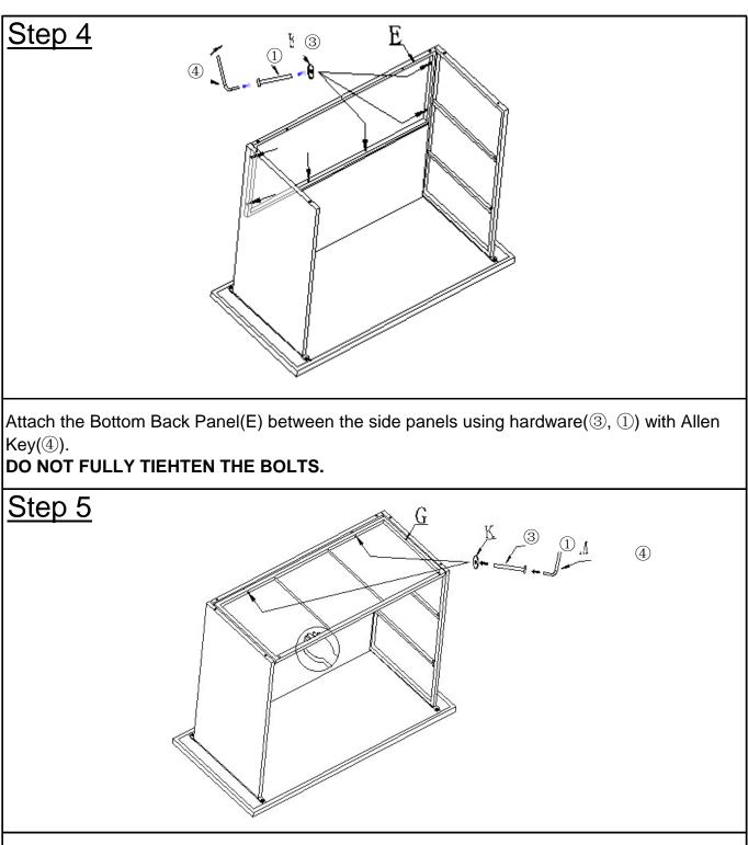
**NOTE: Please have a second adult help you perform the Step 5 & Step 6.** Attach the Bottom Plate(G) to the Bottom Back Panel(E) using hardware(③, ①) with Allen Key(④).
