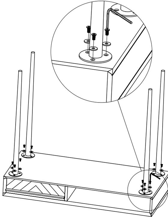
**STEP2** PUT THE WASHERS (H2) ON THE ALLEN BOLT (H1) IN THE ORDER SHOWN IN THE PICTURE
