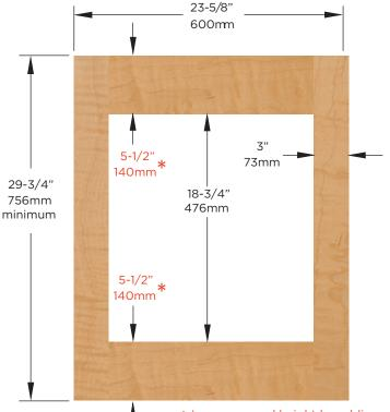
Increase panel height by adding half the increase to both top and bottom. EX: for a 30" panel, Increase 5-1/2" to 5-5/8"
