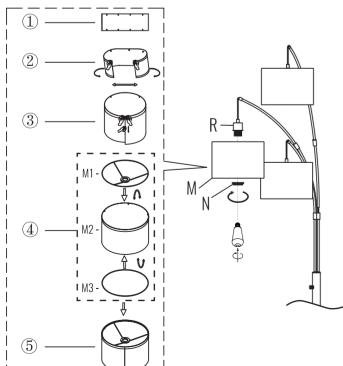
Step 1. Follow the steps ①-⑤ in the illustration to install the shade (M). Step 2. Take down the socket ring (N),Put the Shade (M) into socket (R), then tighten Shade (M) by Ring (N).
