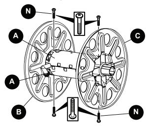
**8.** Ensure the cross brace screws (N) secure both cross braces (A) into the left and right reel sides (B) and (C). See figure below for reference.
