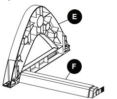
**NOTE:** To disassemble a lower frame bar from a side frame, use a flat head screwdriver to press the lock tab and slide the frame bar out of the snap.
