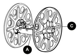
**6.** Align the second cross brace **(A)** tabs with the left and right reel sides **(B)** and **(C)** and assemble as shown.
