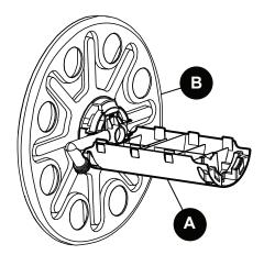
**5.** Align cross brace **(A)** tabs with right reel side **(C)** and assemble as shown.
