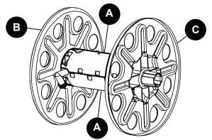
**7.** Using the supplied cross brace screws (**N**) secure cross braces (**A**) to the left and right reel sides (**B**) and (**C**).
