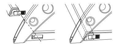
**1.** Align and slide the locking tab on lower frame bar **(F)** with the snap on side frame **(E)** until an audible click sound is heard.
