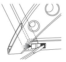
**2.** Align and slide the locking tab on upper frame bar **(G)** with the snap on side frame **(E)** until an audible click sound is heard. Store frame assembly for further assembly.
