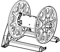
**10.** Install the side frame (E) onto the right reel side (C) and the lower and upper frame bars (F) and (G) as shown.
