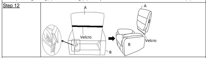
Disassembly Note:open the flap on the Chair Backrest(A),use a screwdriver(Don't use fingers) pressing outward on the metal ear on the preattached Metal Bracket on one side of the Chair Base(B),with assistance of you adult partner to keep the Chair Base(B) in place,pull out the Chair Backrest(A) upward at the same time,repeat the same step for another side. Then the Chair Backrest(A) can be taken out.
