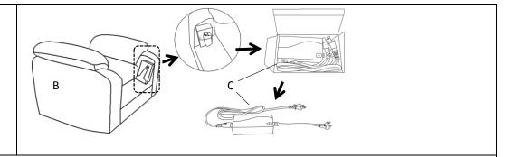
Take out the small carton box and open it to take out the Power Cord with transformer (C).
