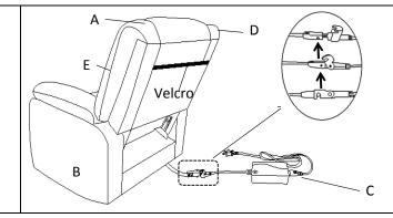
Force apart the draw-ingear , then separate the joint from the motor and Power Cord(C).
