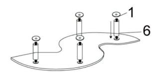
put metal tube(6) on the THREAD(3), and put four WASHER(1) on the MEATAL TUBE(6).
