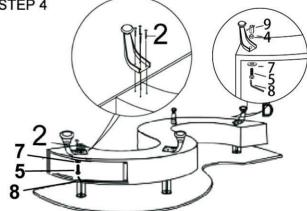
put four table legs(D) on the main structure, then put flat washer(7) on bolt(5), screw four bolts(5) in the big hole of the base(B), put nut(4) on the hole, then use allen wrench(8) tight the bolt(5) screw 16 screws(2) on leg.
