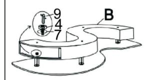
put BASE(B) on the four metal tubes (6), then put four FLAT WASHERS(7) on four holes of BASE(B), and then put four NUT(4) on the FLAT WASHERS(7), then use WRENCH(9), tighten four NUT(4).
