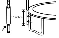
**3.** The set comes with 2 clamps per pole. One being attached 2" **below frame**, while the other being attached 2" **above the end of the lower pole**.
