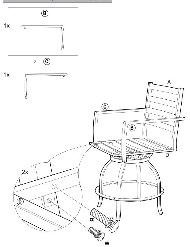
Please ensure A/B/C/D connected well, and then you start to tighten each screw to the end.
