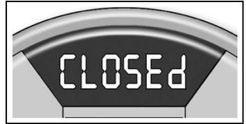
NOTE: The lock design allows for a new user code each time that the safe is locked
