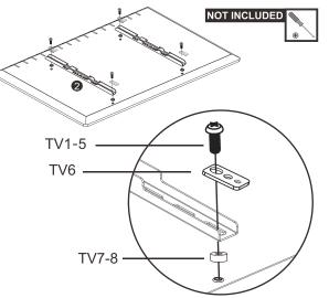
First, make sure the diameter of the bolt ( TV1-5 ) fits your TV. Then, please see the diagram above. You will need to thread the bolt into the TV using the correct washer (TV6) and spacer ( TV7-8 ) if necessary. Please make sure the monitor brackets are vertically centered and level with each other
