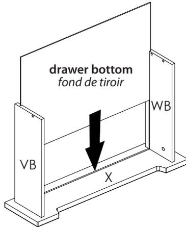
**Drawer bottom must enter into the groove located on panel X**
