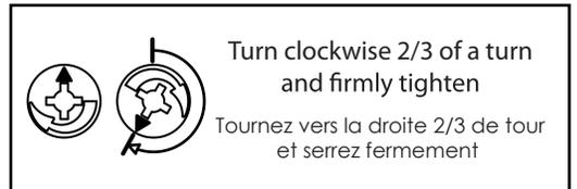
**6** Fasten the panel C to the assembled unit. Then, tighten the 4 cam locks # 0203 located on panels A and B
