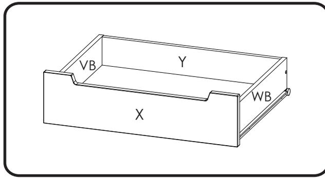
**9** Install 2 small cam locks # 0204 into panels VB and WB. Install 2 push bolts # 2200 into the panel X. Insert 4 wood dowels # 0207 into panels VB, WB and Y
