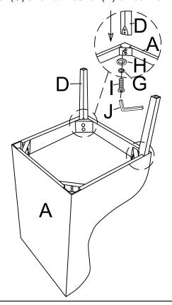
Take the Allen Wrench, and turn the bolts until the legs are secure.
