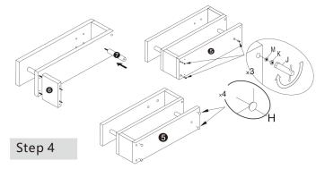
Install the screw rod (P) in the corresponding hole of the table top ① and then install the wooden dowel (E) at the corresponding hole. Then install the connecting board ⑧ at the corresponding hole of the back side from the table top, tighten and fix with spanner (F), screws (B) and metal washer (M).
