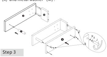
Using the same method as Step 2, assemble the bottom board ⑤, side-support board ⑥ and stainless steel pole ⑦ together. Add on the stick on the waterproof rubber washer H to the bottom of board ⑤.
