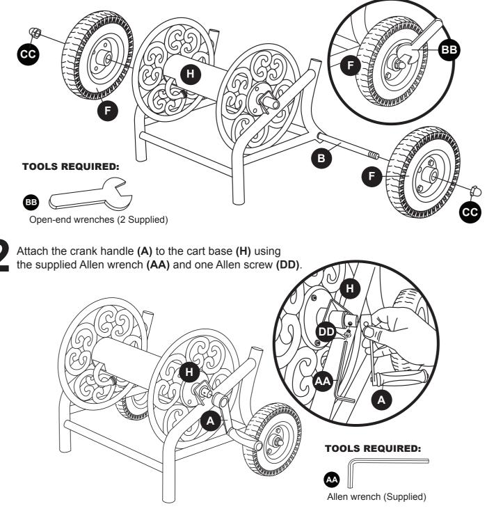
CAUTION: DO NOT OVER TIGHTEN LOCK NUTS AND ALLEN SCREWS.
