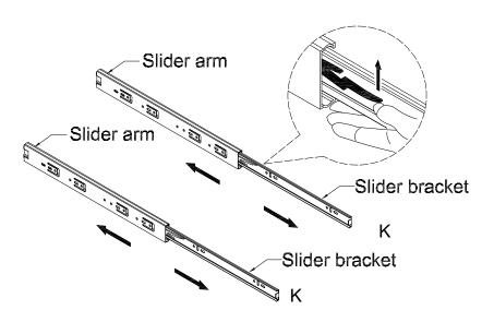
Put slider bracket into slider arm as per diagram.
