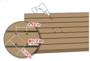
2 Put the baseplate on the deck. Align the four middle holes with the pre-drilled holes.
