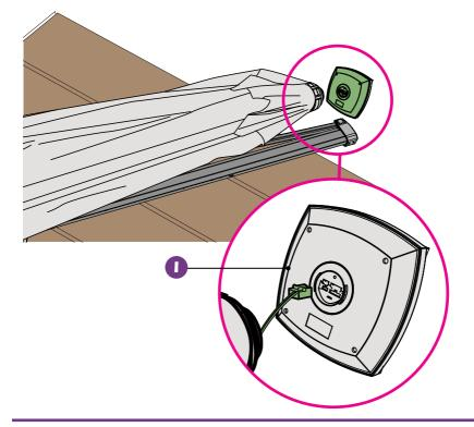
**CAUTION:** The USB cable is used exclusively to charge the battery located on the support arm. There is no need to connect the USB cable to the back of the solar panel.
