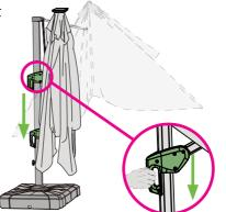
3 Secure the closed canopy to the pole with a strap.
