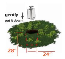
2 Make sure the inground base is horizontal. Backfill the hole with at least 700 lbs of concrete. Concrete >700lbs
