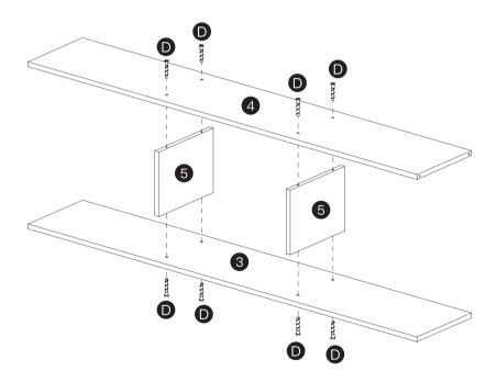
Step 13 Install the part of last step on the frame, use part and to screw them.
