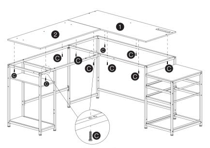
Make sure these screws are throught the holes on the left side.
