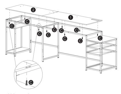
Make sure these screws are throught the holes on the left side.
