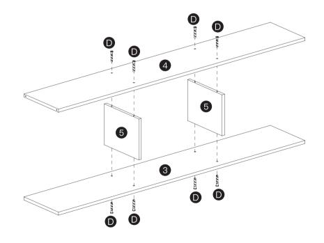
Step 13 Install the part of last step on the frame, use part C and D to screw them.
