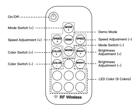
NOTE: To use the remote control, it must be pointed directly at the sensor on the light strip.
