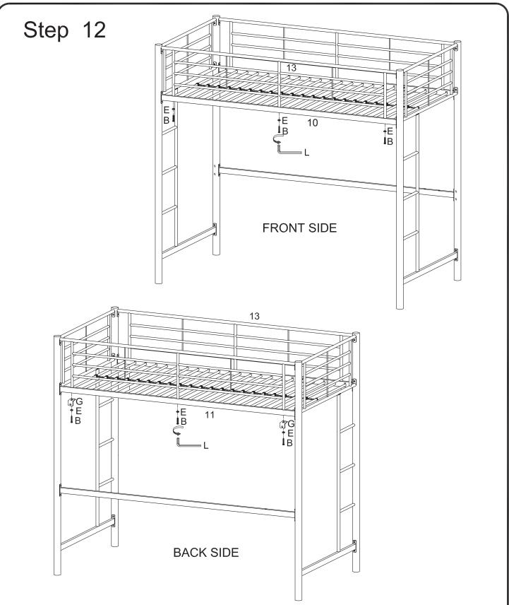
Secure front guardrail (13) to crossbar (10) using large bolts (B) and large washers (E). Secure back guardrail (13) to crossbar (11) using large bolts (B), large washers (E) and, where applicable, angle brackets (G).\* Tighten large bolts (B) with large wrench (L).
