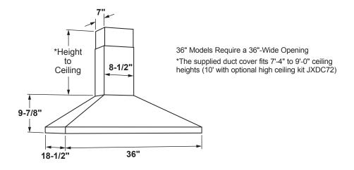
The vent hood must be installed 24" min. above the cooking surface. For optimal performance, installing the hood more than 38" above the cooking surface is not recommended. The hood installation height above the cooking surface depends upon ceiling height. The telescopic duct cover conceals the ductwork running from the top of the hood to the ceiling.
