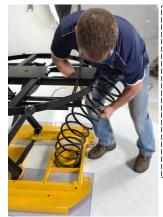
Spring properly seated inside receiver and plug reinstalled.
