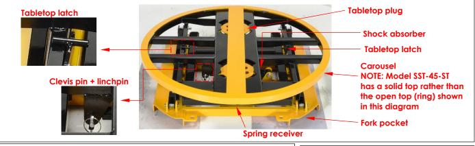
**Step 1**: Remove the (yellow) carousel from the tabletop. Then, remove the linchpin and clevis pin to release one end of the shock absorber from the shock bracket as shown below.
