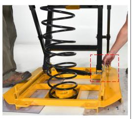
**Step 7**: Press the tabletop down until the latches catch; then pull out the free end of the shock absorber and attach it to the shock bracket using the clevis pin and linchpin.
