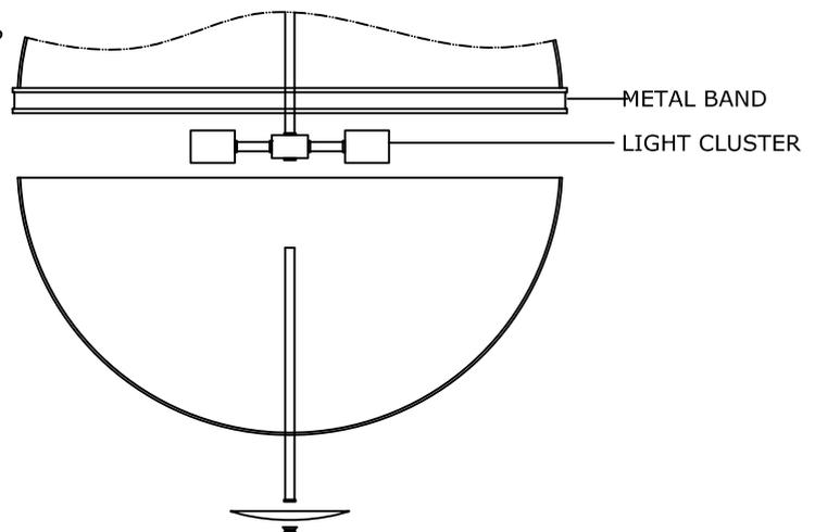
NOTICE: TO REPLACE THE BULB, PLEASE UNSCREW THE BOTTOM FINIAL FROM BOTTOM METAL CAP AS SHOWN ABOVE
